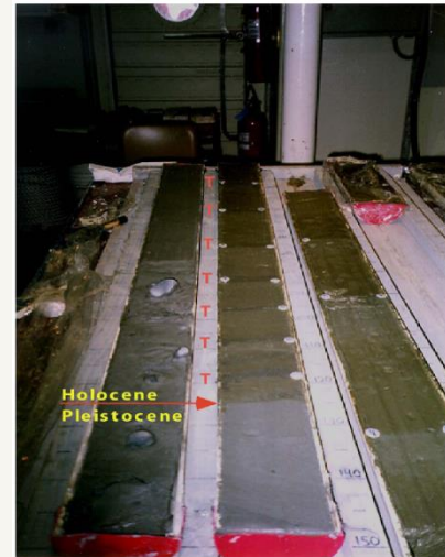
Figure 2-47. Deep Sea Sediment Cores that Record Past Megathrust Earthquakes off the Oregon Coast
