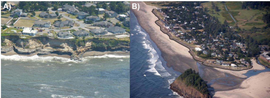
Figure 2-32.(A) Houses Line the Cliff at Fogarty Creek in Lincoln County. (B) Extensive Erosion along the Dune-Backed Beaches in Neskowin Have Resulted in the Construction of Massive Riprap
