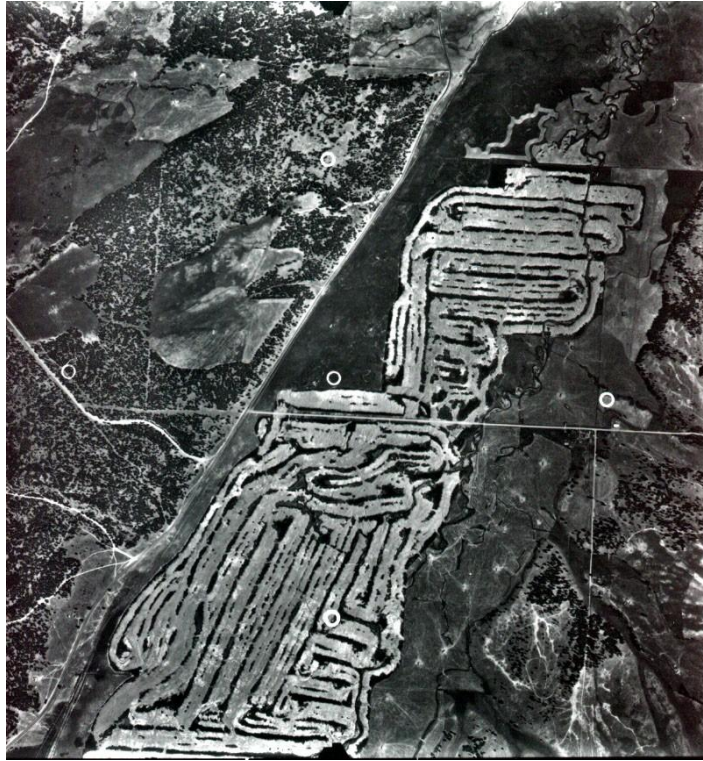
Figure 3-5. LIDAR aerial photograph of Sumpter Valley floodplain restoration site showing ponds and rows of gravel deposits created by dredging (Powder Basin Watershed Council 2011).
