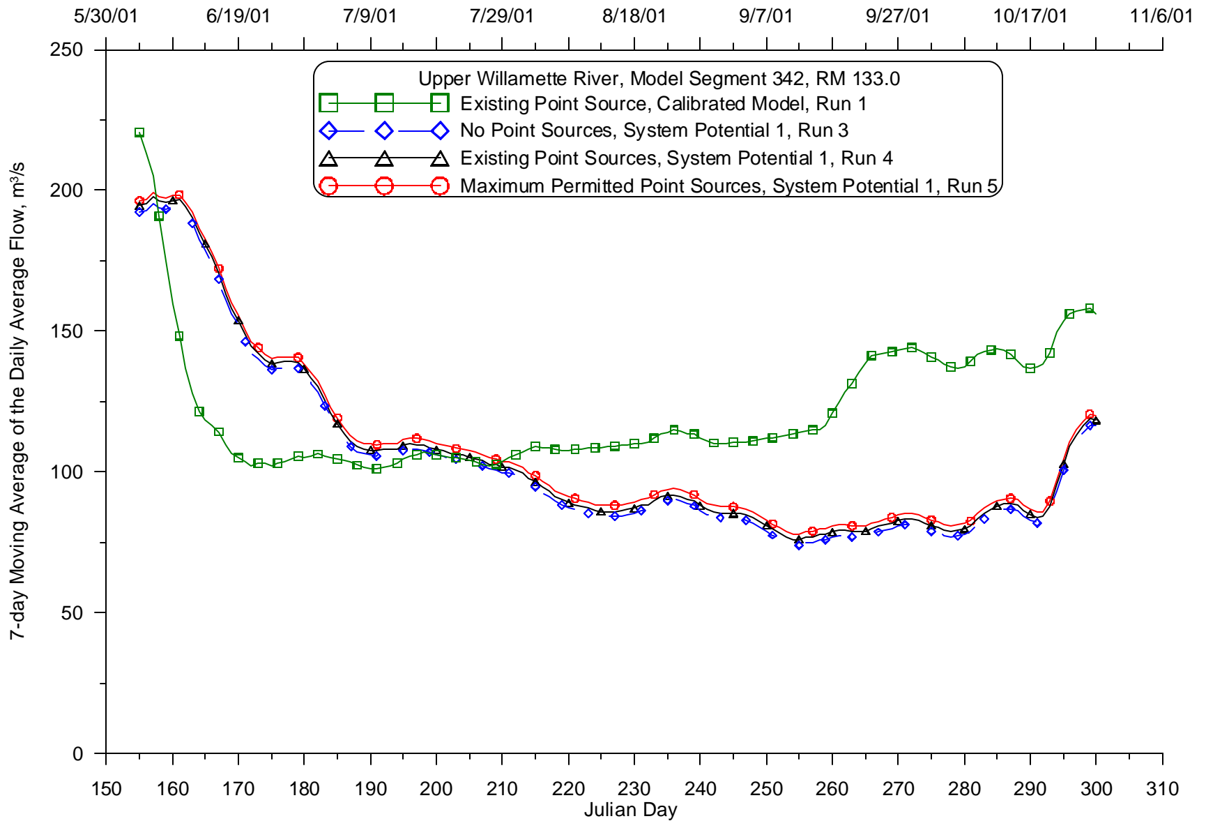
Figure 96: Calibrated model and System Potential 1 (varying point source discharges) 7-day moving average of the daily average flow comparison for 2001 for the Willamette River at RM 133.0
