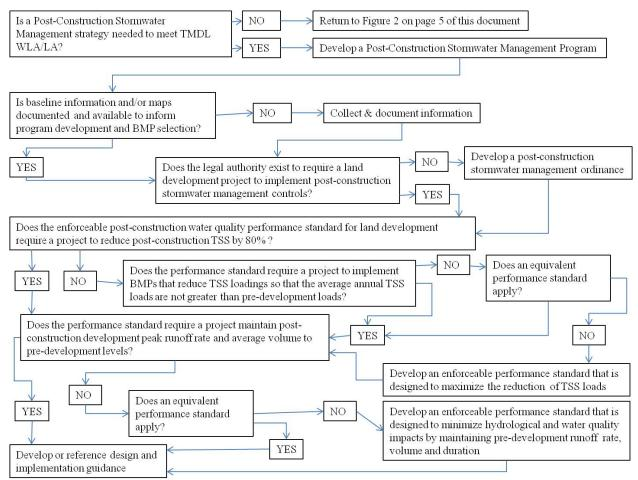
Figure 4 – Stormwater Post-Construction Program Development Flowchart
