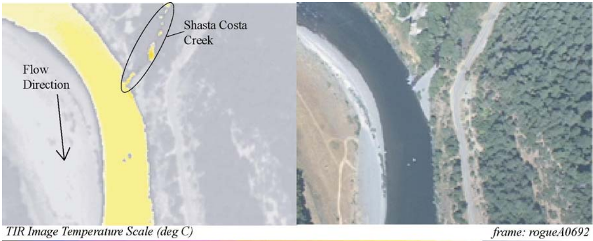
TIR/color video image pair showing the confluence of Shasta Costa Creek (24.4°C) to the left bank of the Rogue River (25.4°C) at river mile 28.8.
