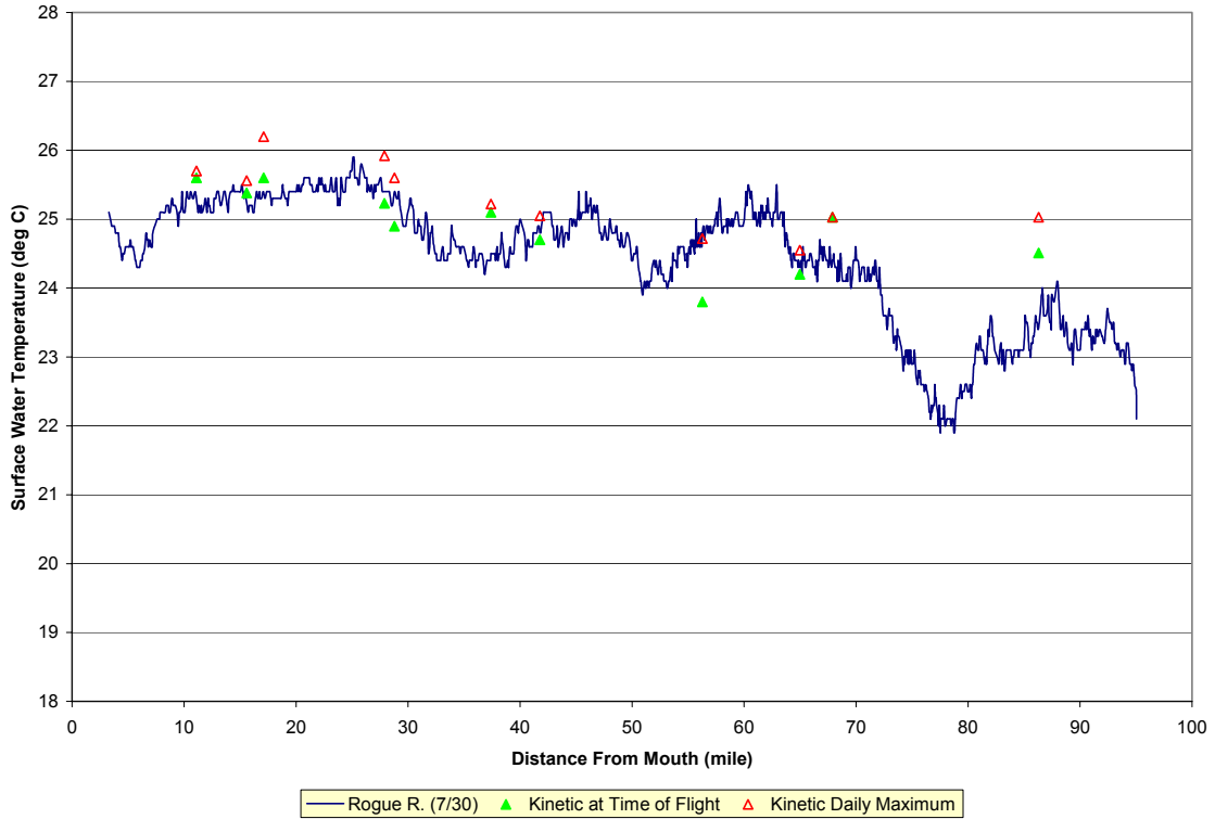
Figure B-1 – Median channel temperatures versus river mile for the Rogue River, OR, on July 30, 2003.
