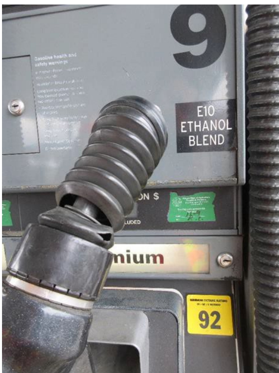
(AQGP-23) Balance System- bellows torn
