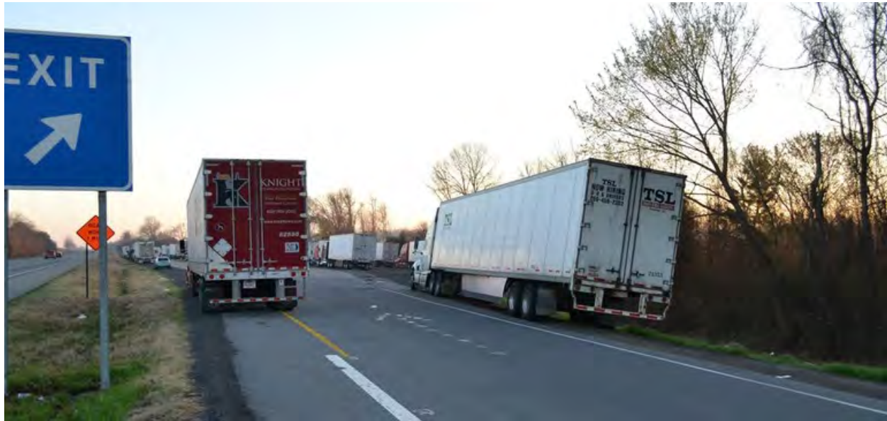
Figure 6: Undesignated Parking Near a Truck Parking Stop
