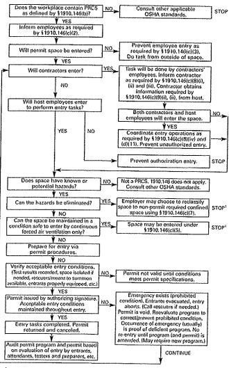
Spaces may have to be evacuated and reovaluated if hazards arise during entry. Source: 29 CFR 1910.146 Appendix A.
