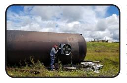
In April, at the Department of Public Safety Standards and Training's (DPSST) facility in Salem, an ammonia railroad housing was welded to the side top of a DOT111 training prop car (a retired railcar installed through the HazMat by Rail program in 2017). The welding project enhancement allows for firefighters to train on different types of rail housing which require various equipment, including the Midland Kits.
