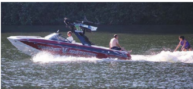
Riding on the transom of a boat that's underway is dangerous – for falling overboard and possible CO poisoning and it is illegal.
