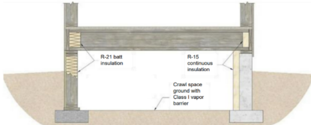
Figure 1: The most straightforward of these options is to make the under-floor space part of the thermal envelope.
