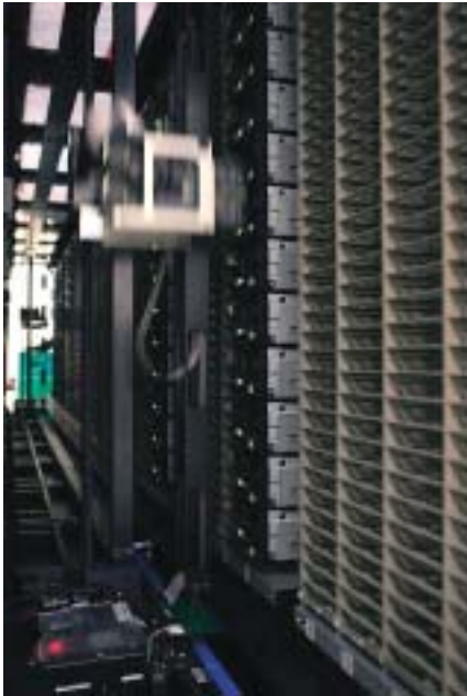
Two robotic arms insert and eject tapes into the library
