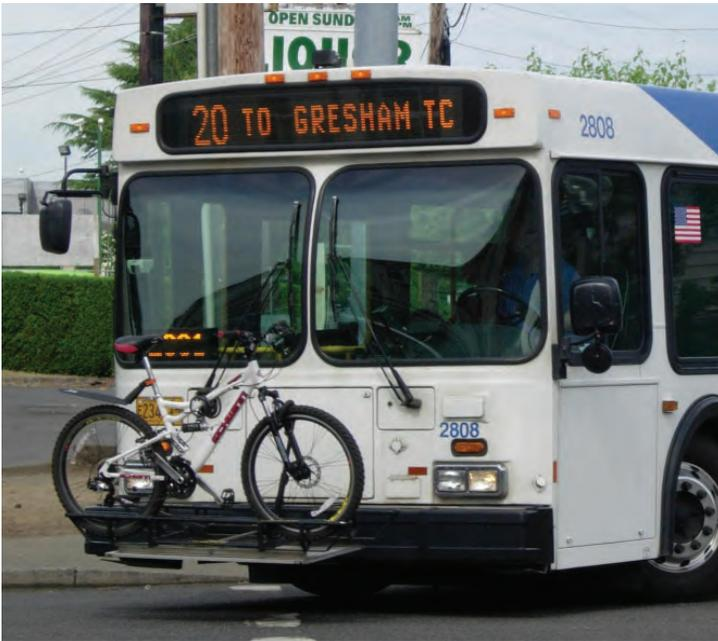
TriMet offers an example of connecting the bicycle and transit networks by allowing cyclists to load bikes on its buses, trains, and streetcars.
