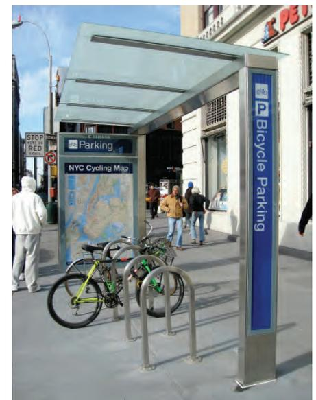
This bike station uses simple staple racks and provides shelter.
