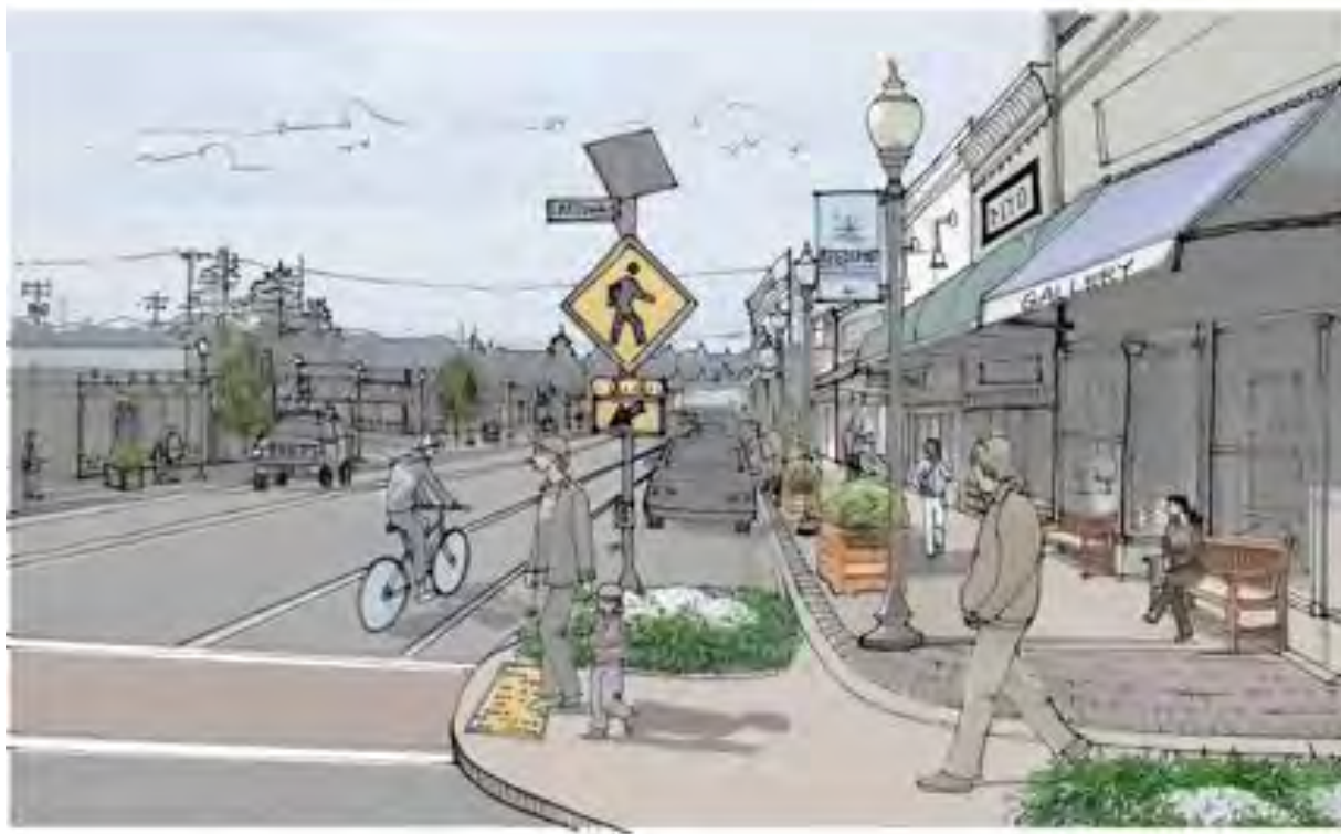
Figure 14 gives a typical downtown street section with curb extensions that “shadow” or match parallel parking width.
