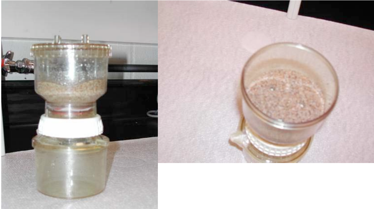
Figure 5: Experimental set-up for measuring the rate of Cd release from fertilizer in moist sand.
