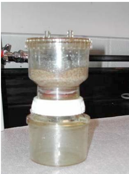
Fig. 3. Apparatus for studying dissolution of Cd from fertilizer particles.
