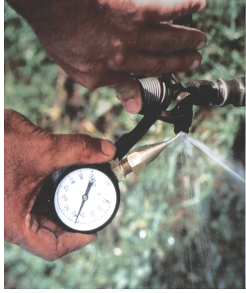
Checking nozzle pressure
