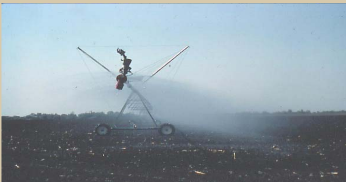
Chemigating when the wind speed exceeds 10 mph may result in crop damage from wind drift.
