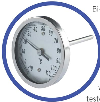
Bi-metal thermometers (as shown in the picture to the left) are not designed to measure the temperatures of thin foods, and can only be used for foods like soups, roasts, or tuna salad.
