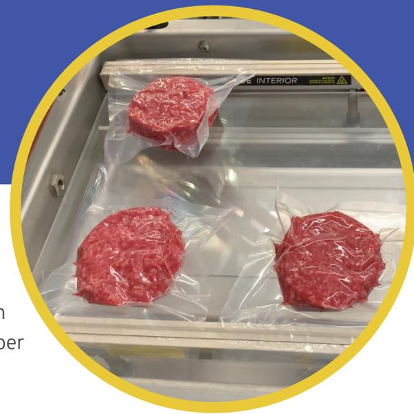
Reduced Oxygen Packaging (ROP) is done in many ways. The most common use of ROP in a food establishment is to mechanically remove air from around food in a plastic bag to create a tight seal, which is also called vacuum packaging. Packaging food in resealable zipper storage bags is not considered ROP.
