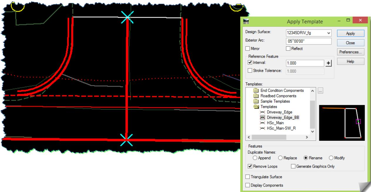
17) Use the **GENERATE SLOPED SURFACE** tool to create a **1 : 4** daylight slope grading similar to the earlier driveway modeling.
