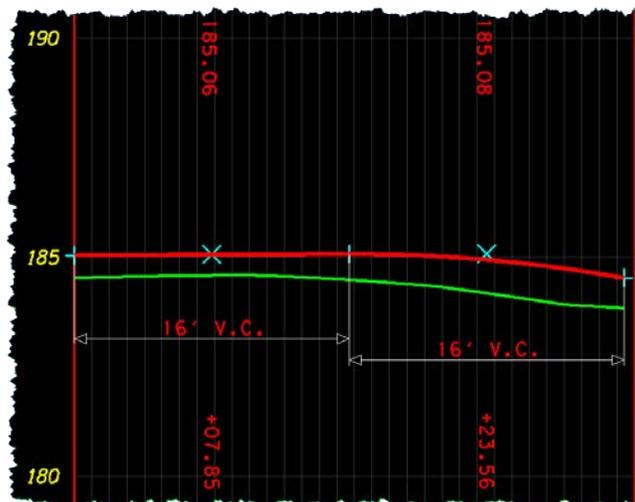
10) Import the returns into the FG surface using **IMPORT SURFACE > FROM GEOMETRY**.
