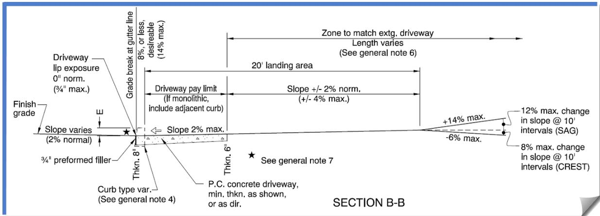
The layout of this type of driveway is very similar to the first driveway in this module, except that this one has a slightly simpler configuration due to the parallel nature of the front and back of the sidewalk; however it has added complexity due to the maximum criteria that must be met.
