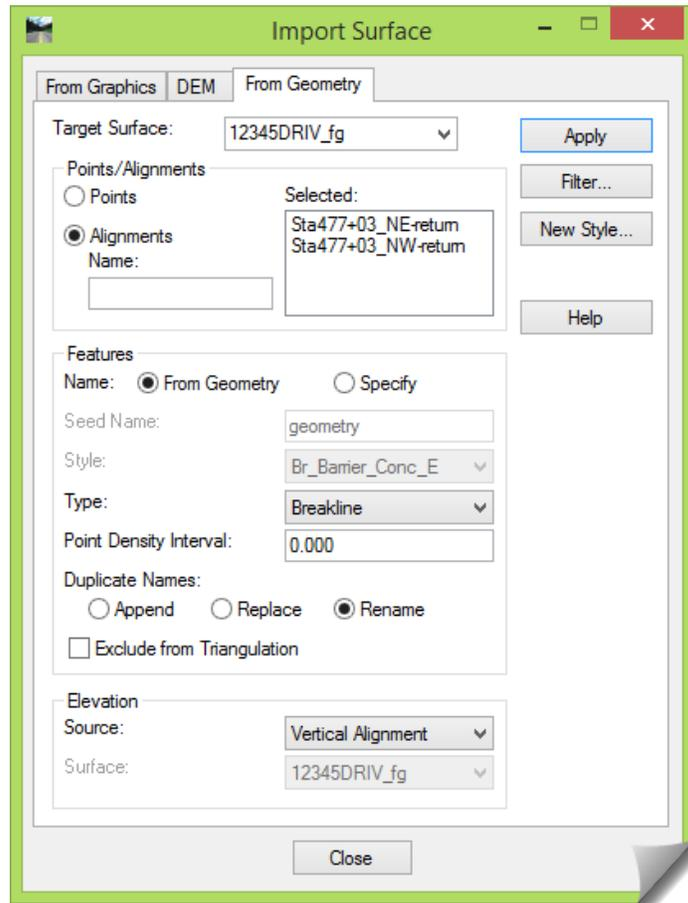
11) **DELETE** the graphics for the geometry returns as well as the 20' parallel guide lines, and view the new surface **Features** for those same elements to verify that they have been created and now exist in the surface model.
