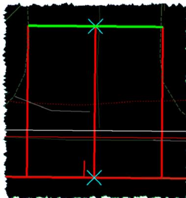
The **MULTICENTER CURVE** tool will be used to create the curve returns for each side of the approach. This tool is fairly intuitive and the diagram explains the settings that are required for the construction and execution. Not only does this tool create the **Horizontal** alignment for the return based on the settings on the **MAIN** tab, it can also create the **Vertical** alignment per the settings on the **ADVANCED** tab.
