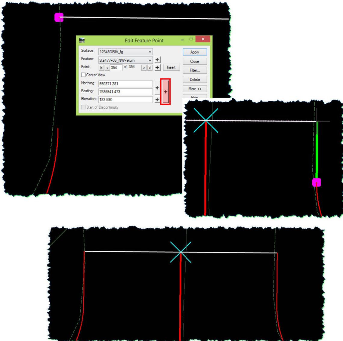
Now a partial template will be run around the radial returns and back toward the approach tie-in edge along the back. This template will be run without the Cut / Fill slopes.
