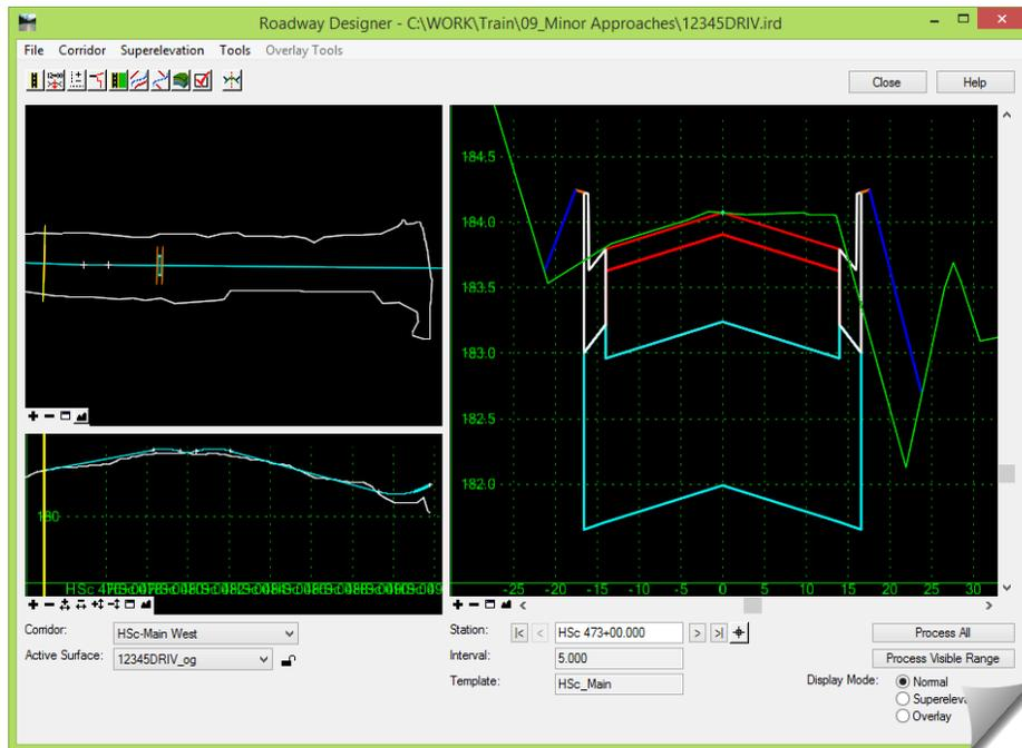
There is only one **Corridor** in the **ROADWAY DESIGNER**, **HSc-Main West**. This **Corridor** was used to create the FG design surface.
