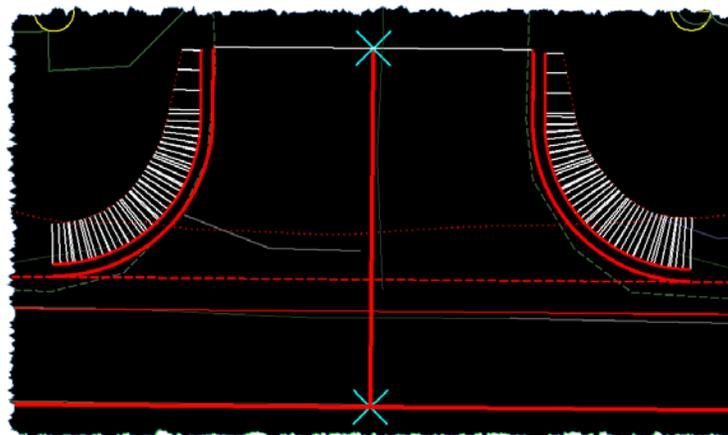
Because an isolated curb template was used without the roadway connected to it, the Feature **CurbBF-S\_L** became integrated into the triangulation. This will have to be excluded.
