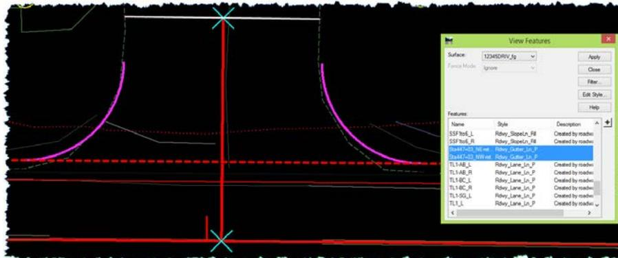
There are a number of ways to perform this next step. The desired result is to develop a breakline from the end of the return to the approach tie-in. A few options would include moving the last point on the return, inserting a new point on that breakline, or using the **PLACE FEATURE** tool.
