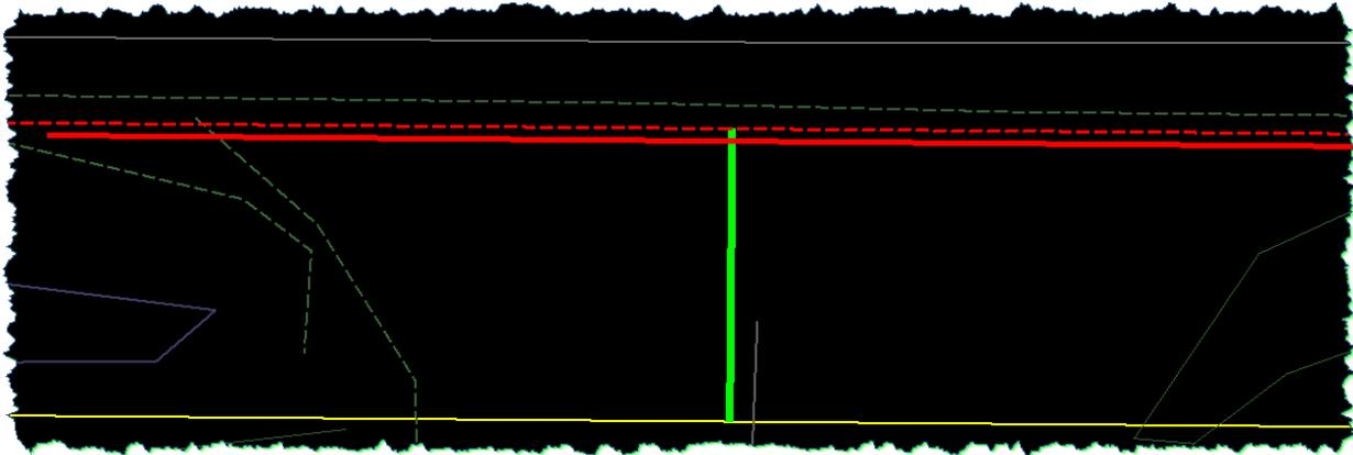
Now some construction elements will be created for the key driveway widths. These will be used later as guide lines and key points for snapping.
