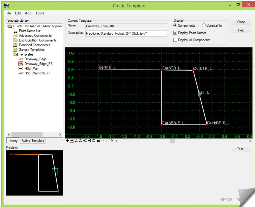
16) Using **APPLY TEMPLATE**, run this template around both approach edges.
