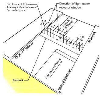
Figure 5: Vertical Illuminance measuring Grid at Mid-block Crosswalk
