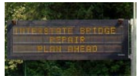
Changeable message signs (CMS) located in strategic locations along highways provide information to motorists about potential delays ahead.
