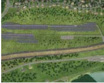
Artist's conception shows a solar array installed next to a highway to provide power for lighting.
