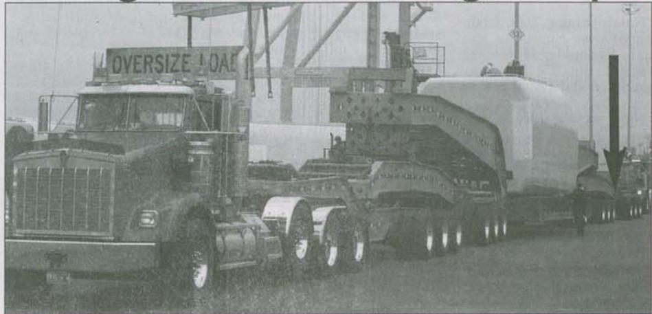
ARROW SHOWS the end of the extremely large truck system Wilhelm Trucking and Rigging Co. of Portland needed to transport a wind tower nacelle up Interstate 84 on its way to Ellensburg.
