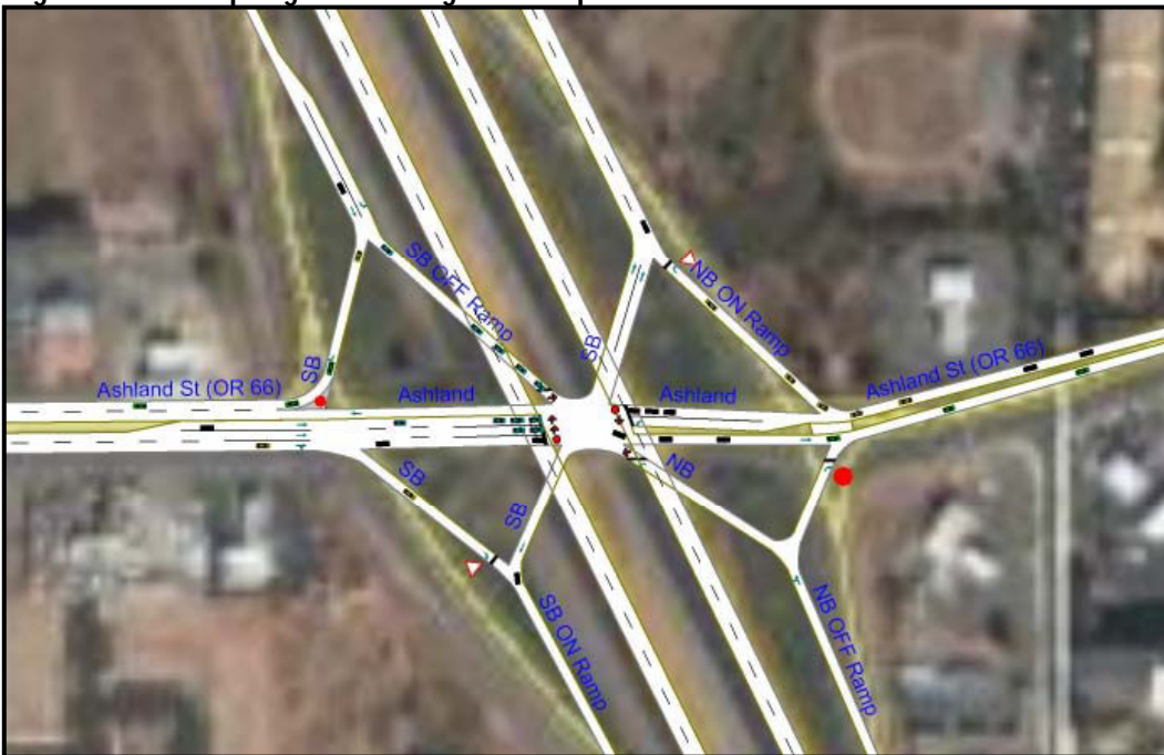
Figure 8. Green Springs Interchange Build Option 14-4: SPUI
