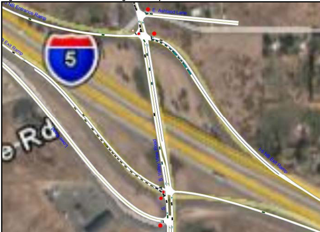
Figure 9. North Ashland Interchange Build Option 19-1
