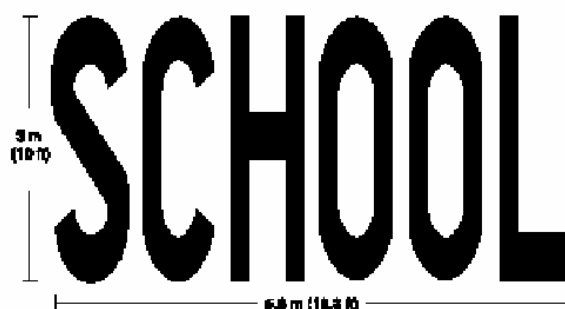
Figure 7C-1. Two-Lane Pavement Marking of "SCHOOL"
