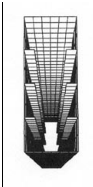
Figure 2.13: End view of finite element model used to estimate thermal stresses in flange of box girders
