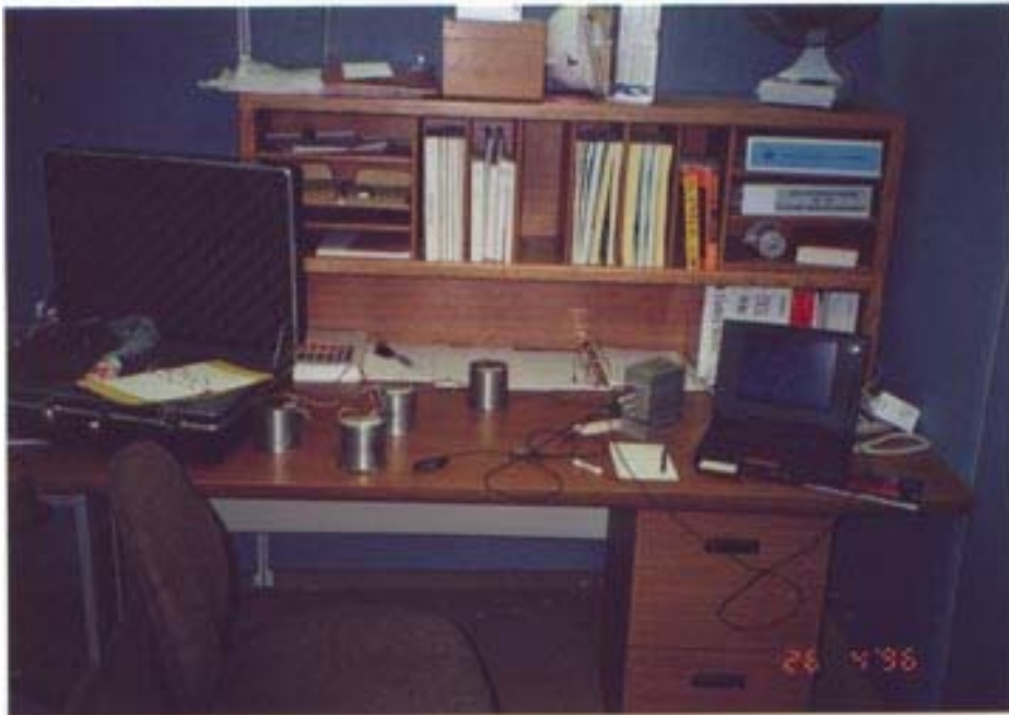
Figure 2.17: Weld metal core strain measurements. Top photo shows gauge reading prior to core removal and bottom photo shows strain measurements after cores were removed from flange ESW.
