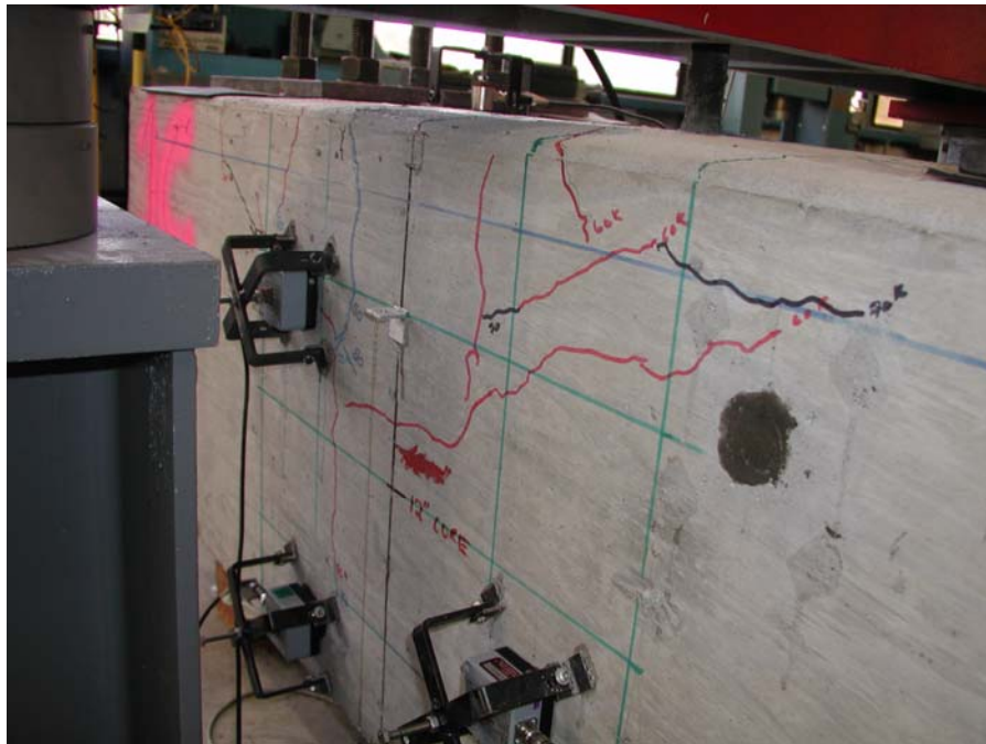
Figure 2.29: Picture of Specimen 1M12.21 near failure, with cracking observed
