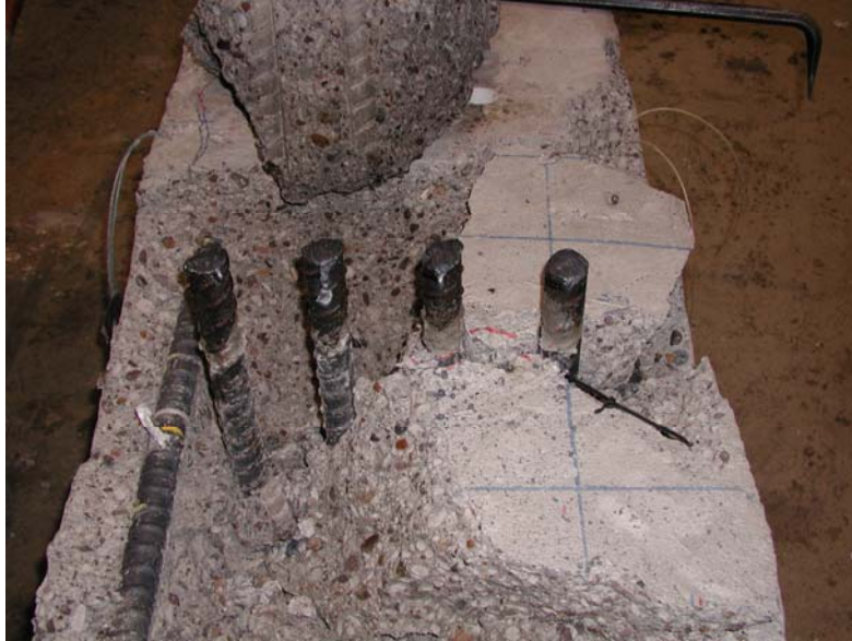
Figure 2.20: Failure of Specimen with concrete wedge, bar imprint visible
