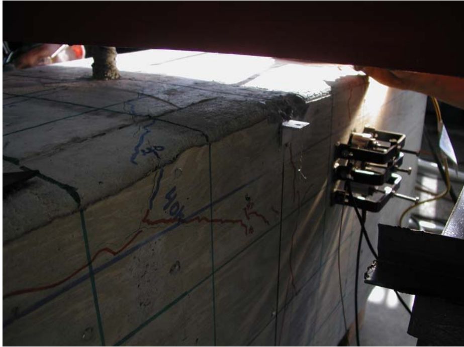
Figure 2.28: Picture of Specimen 1M08.21 prior to failure, with cracking observed
