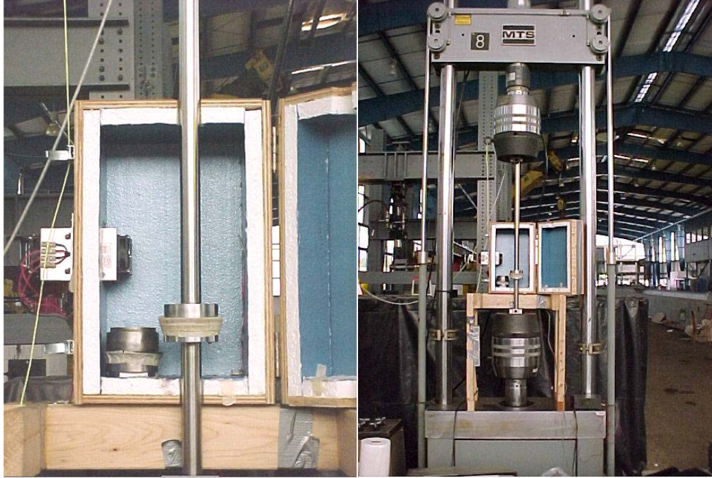
Figure 2.2: Arrangement of the test fixtures in the temperature chamber and in the fatigue machine
