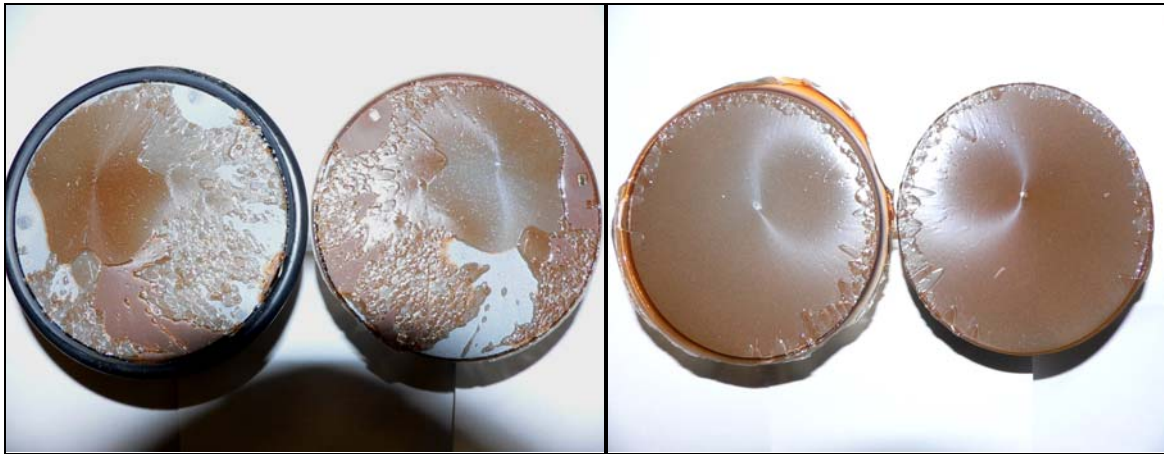
Figure 3.1: Fracture surfaces of static (left) and cycled (right) specimens from run 10 in Table 3.1.
