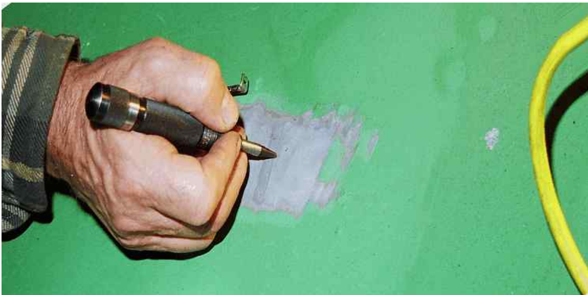
Figure 20 (71149-08) Punch marked weld
