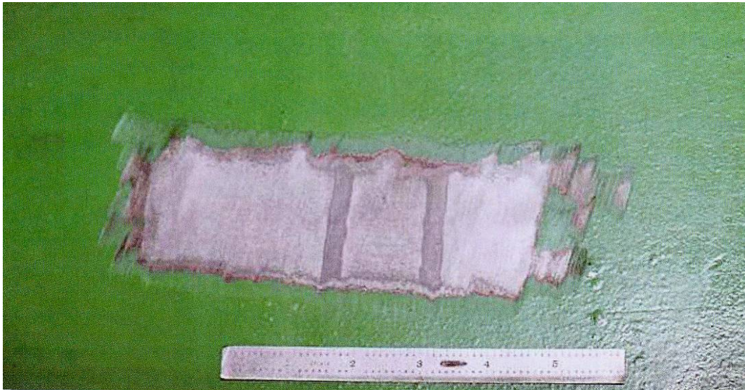
Figure 4.2: Etched ESW showing fusion lines prior to core removal
