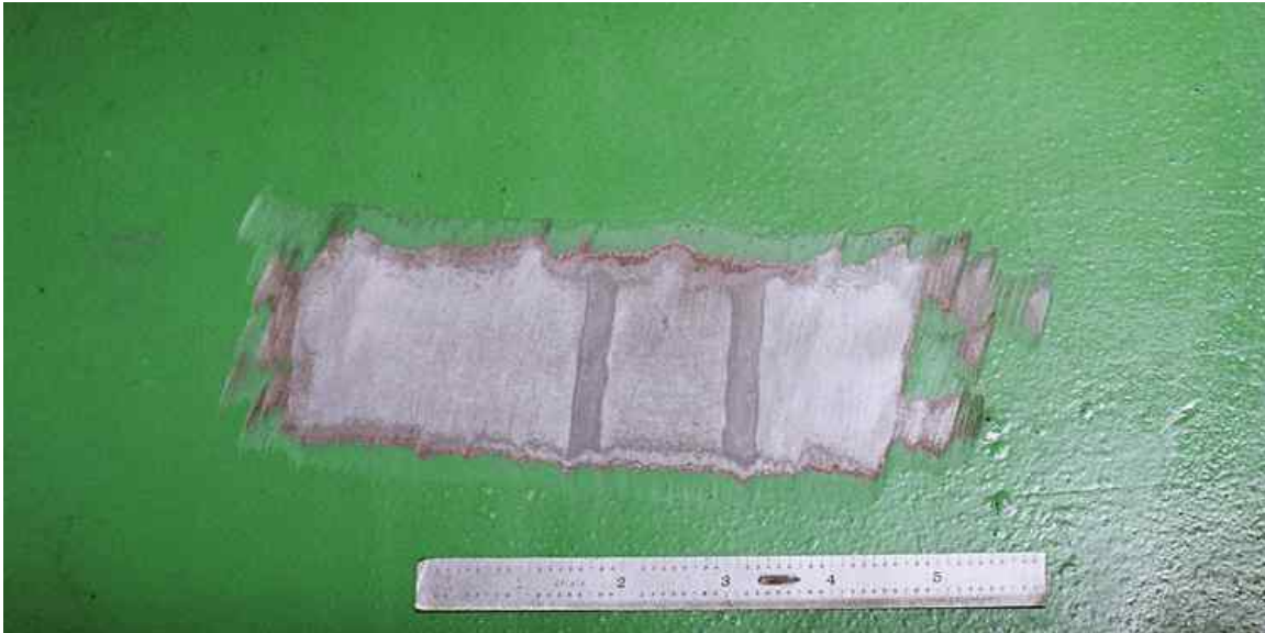
Figure 19 (71149-07) Etched weld (10% Nital)
