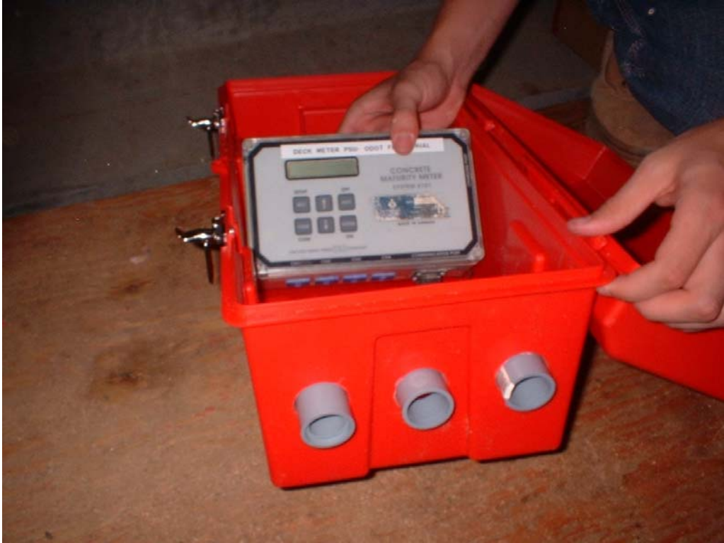
Figure 3.3: Protection of the maturity meter
