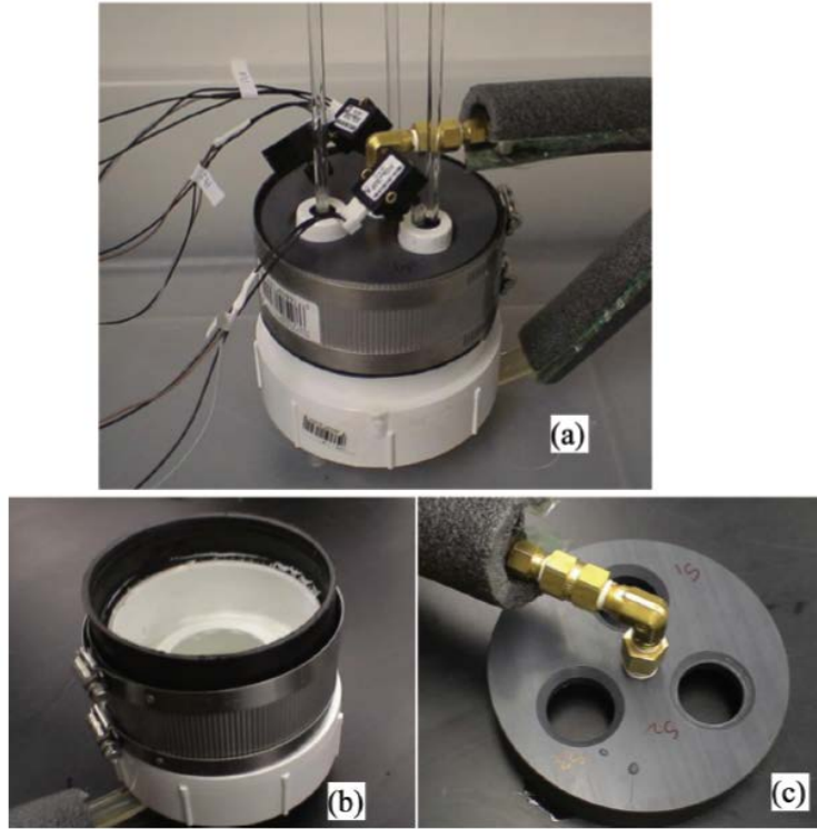
Figure 4.12: Pressure method device to measure chemical shrinkage: (a) whole assembly; (b) main chamber; (c) closure (Peethamparan et al. 2010)
