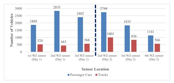
Figure 5.1: Traffic volumes for different vehicle types recorded by active WZ sensors for day 1 (blue lights on) and day 2 (blue lights off) (Case Study 1)
