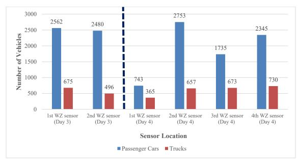
Figure 5.2: Traffic volumes for different vehicle types recorded by active WZ sensors for day 3 (blue lights off) and day 4 (blue lights on) (Case Study 1)
