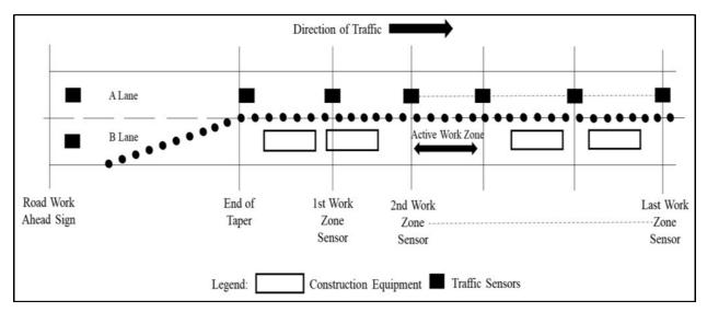
Figure 4.3: Typical sensor placement plan in work zone
