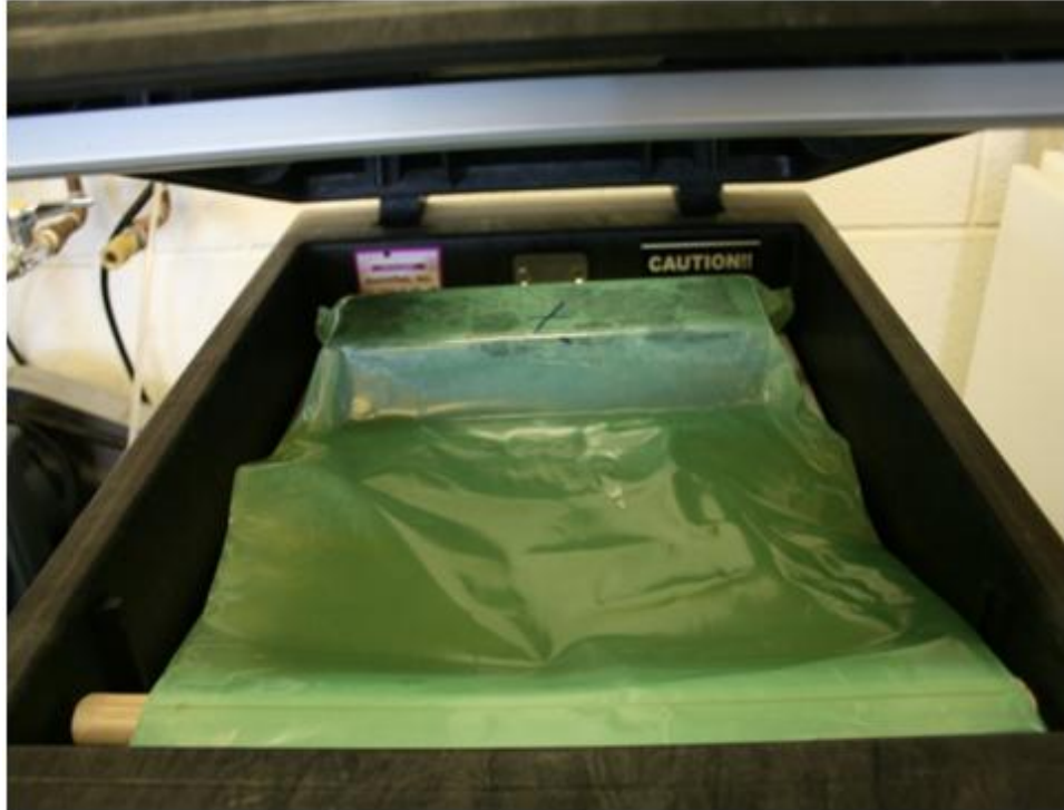
Figure 4.16 - Vacuum Seal Process Complete
