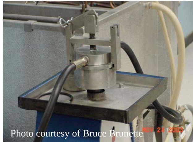
b) Test Chamber in Shaker
