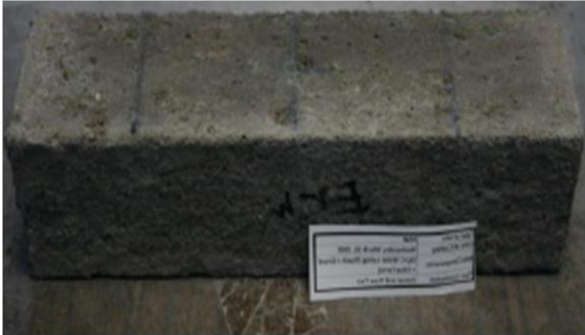
Figure 5.3 - Surface Scaling Evident on Experimental Mixture with Fly Ash (ECW)
