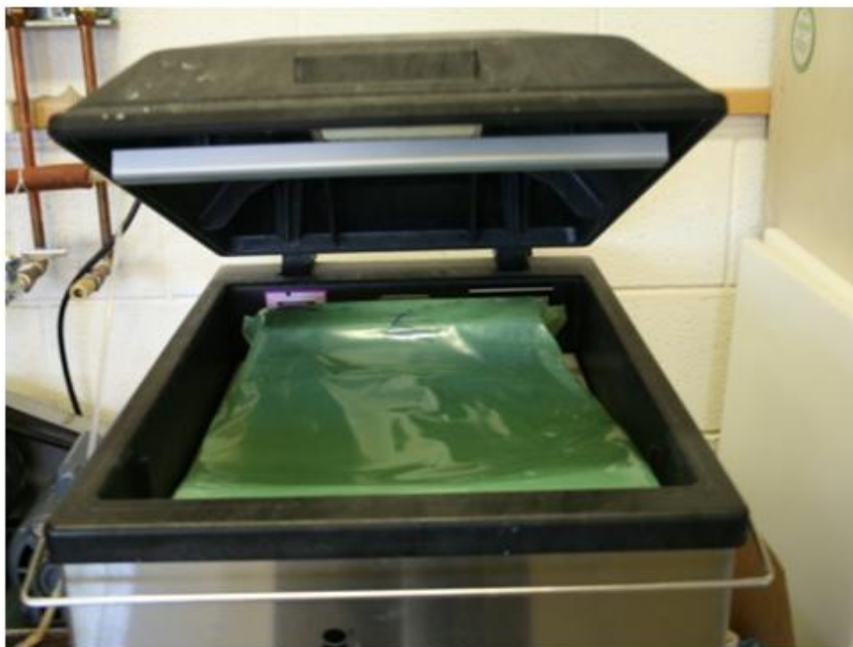
Figure 4.15 - Ready for Vacuum Seal Process
