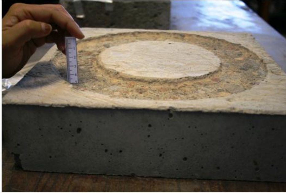
Figure 4.6 - Abraded Surface After Test Showing Depth of Abrasion
