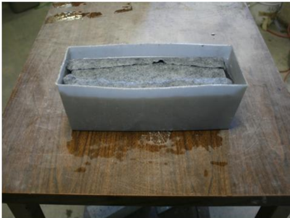
Figure 4.13 - Wrapped Specimen Submerged in Water
