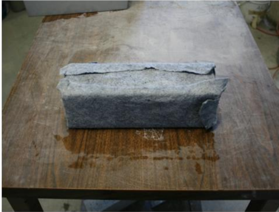
Figure 4.12 - Specimen Wrapped in Felt
