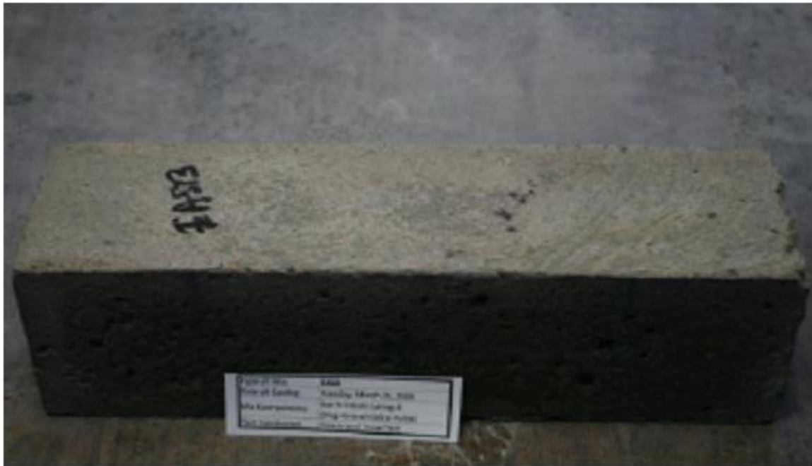
Figure 5.4 - Surface Scaling not Evident on Experimental Mixture with Slag (EASB)
