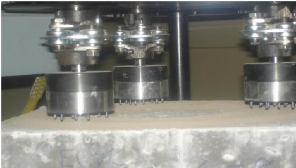
Figure 4.3 - Revolving Disks with Tungsten Carbide Studs
