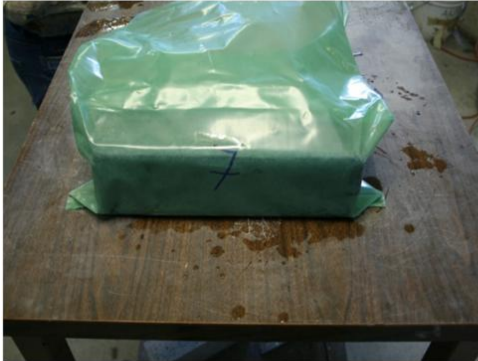
Figure 4.14 - Wet Specimen inside Vacuum Seal Bag
