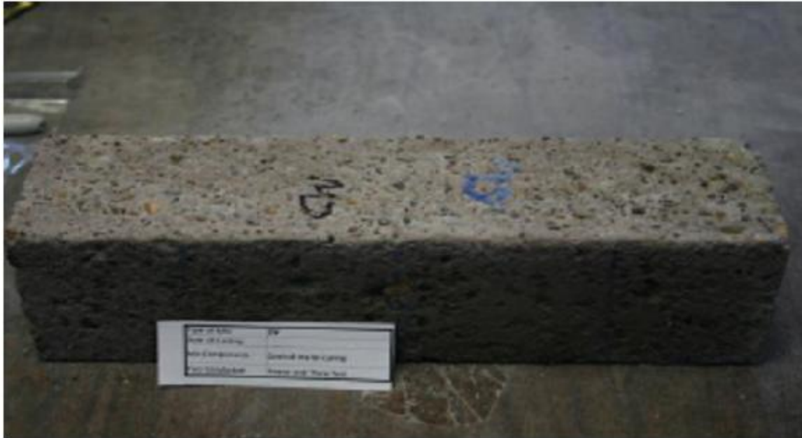
Figure 5.1 - Surface Scaling on the Control Mixture Specimen (CW)
