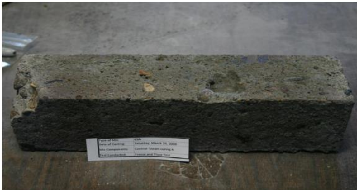
Figure 5.2 - Broken End on Control Mixture Specimen (CSA)
