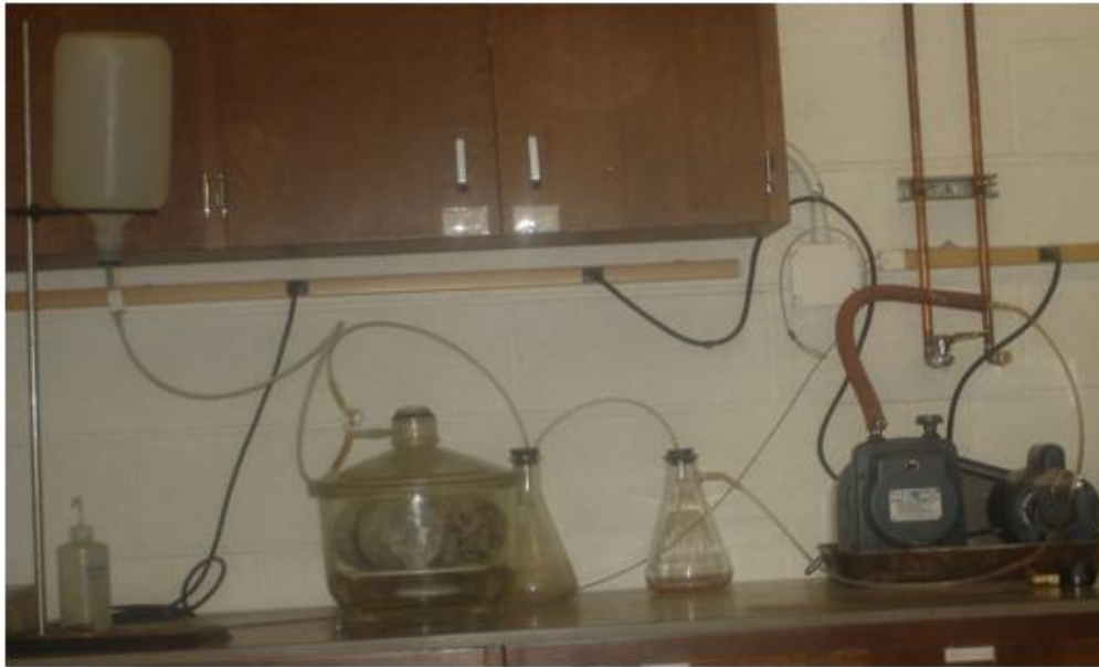
Figure 4.9 - Setup for Conditioning the Specimen
