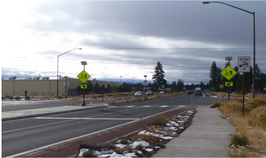
Figure 3.4 Driver's perspective of RRFB installation at the Bend Parkway and Badger Road
