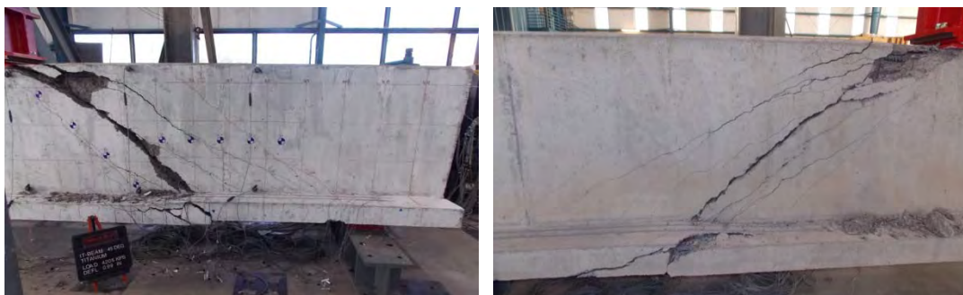
Figure A.8 – Specimen IT.45.Ld3(10).Ti front and back failure photographs
