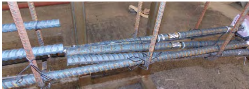
Figure D.13 - Midspan reinforcing steel terminations for Mosier specimens
