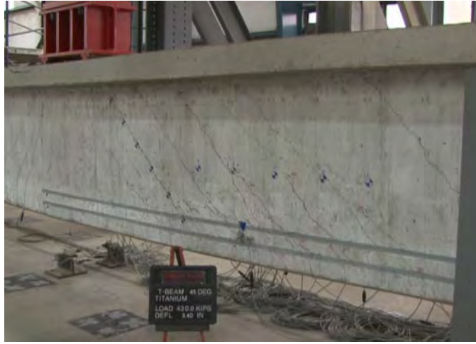
Figure B.31 - Specimen T.45.Ld3(6).Ti at failure
