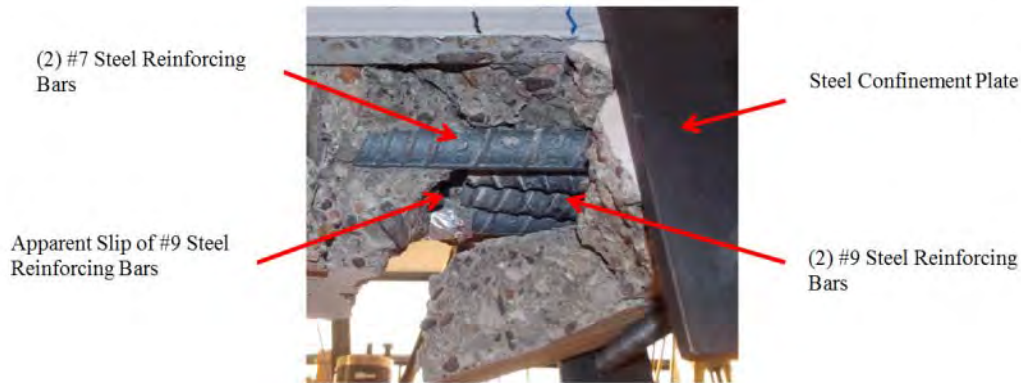
Figure D.28 - Apparent slip of #9 Steel Reinforcing Bars in Mosier 3.
