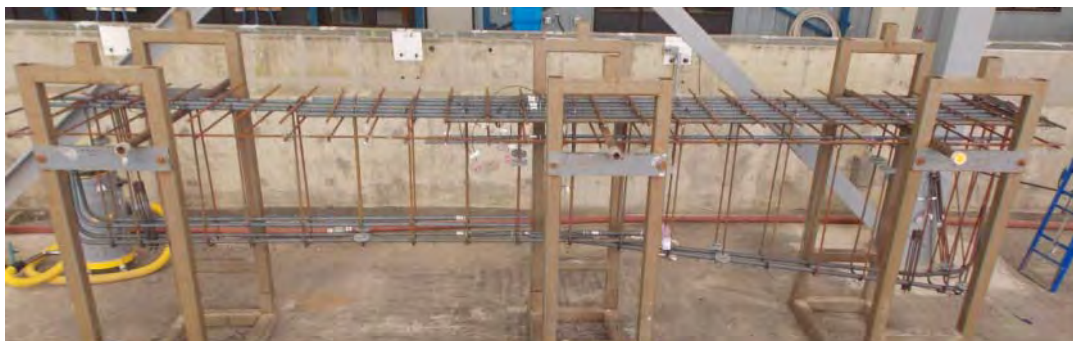
Figure D.14 - Mosier 1 reinforcing steel cage
