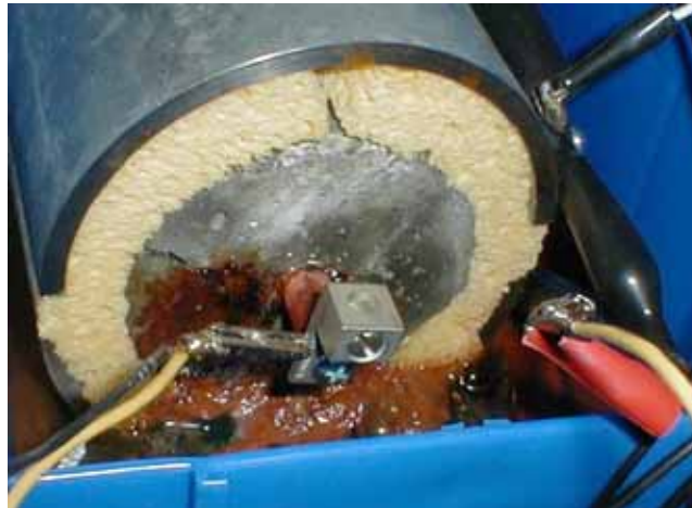
Figure 2.3: Accelerated corrosion of reinforcing steel in a small concrete cylinder. Wetted sponges surround the concrete cylinder and provide electrical contact to steel anodes surrounding the entire assembly.
