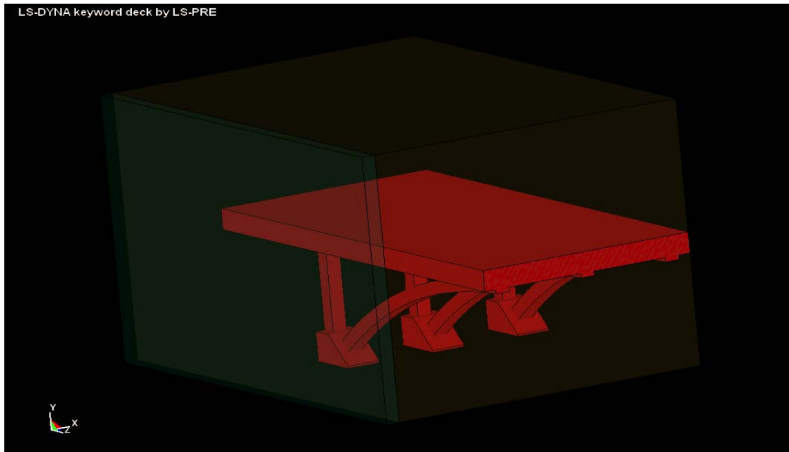
Figure 22. 3D model of the bridge; the box enclosing the bridge is rendered transparent; the box itself contains two parts: one with dark green color is air, one with light blue color has water for introducing the tsunami.
