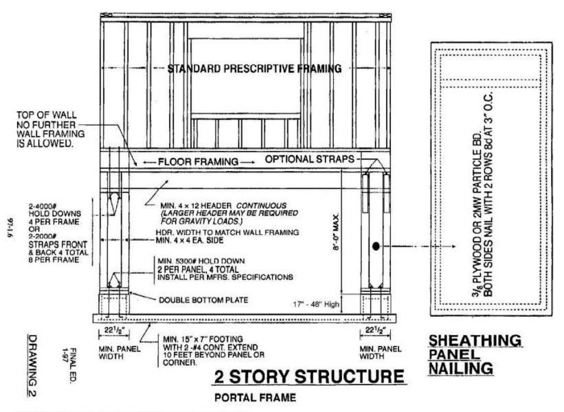
NOTE: Portal frames are allowed by prescriptive construction, only on the first floor of one and two storied structures. NOT ALLOWED IN THREE STORIED STRUCTURES.
