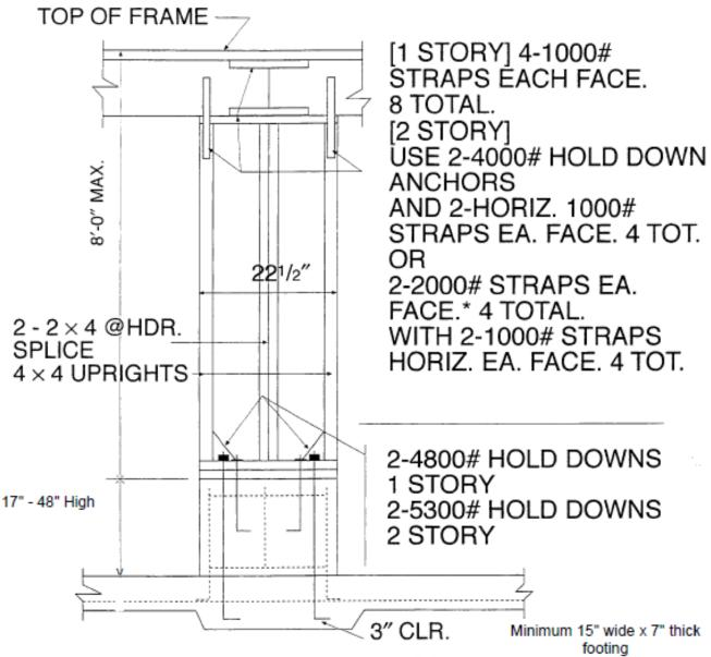
SEE PORTAL FRAME DRAWINGS FOR FOUNDATION, HOLD DOWN AND PLYWOOD NAILING.
