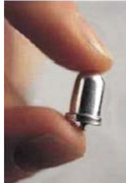
Mercury switch for vehicle convenience light.
