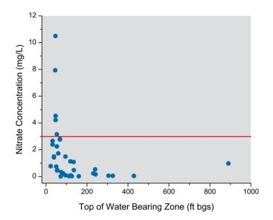
Figure 3. Nitrate concentration and depth to top of the water bearing zone for wells where well log information was available. Red line indicates a concentration of 3 mg/L, which DEQ considers to be an elevated nitrate concentration.
