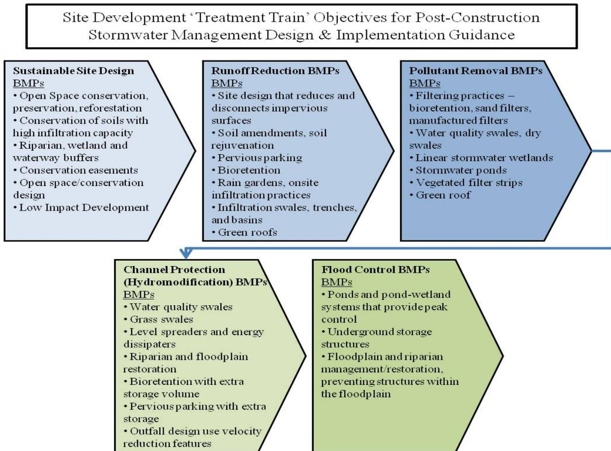
Figure 5 – Post-Construction Stormwater Management 'Treatment Train' Concept
