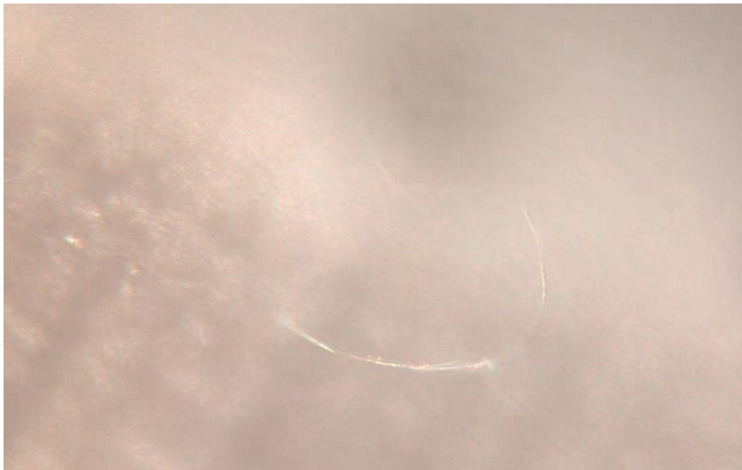
Figure 8: CFU118 -R1 showing a \geq 100 \mu\text{m} vitreous fiber recovered from Field 92 (Table 2).
