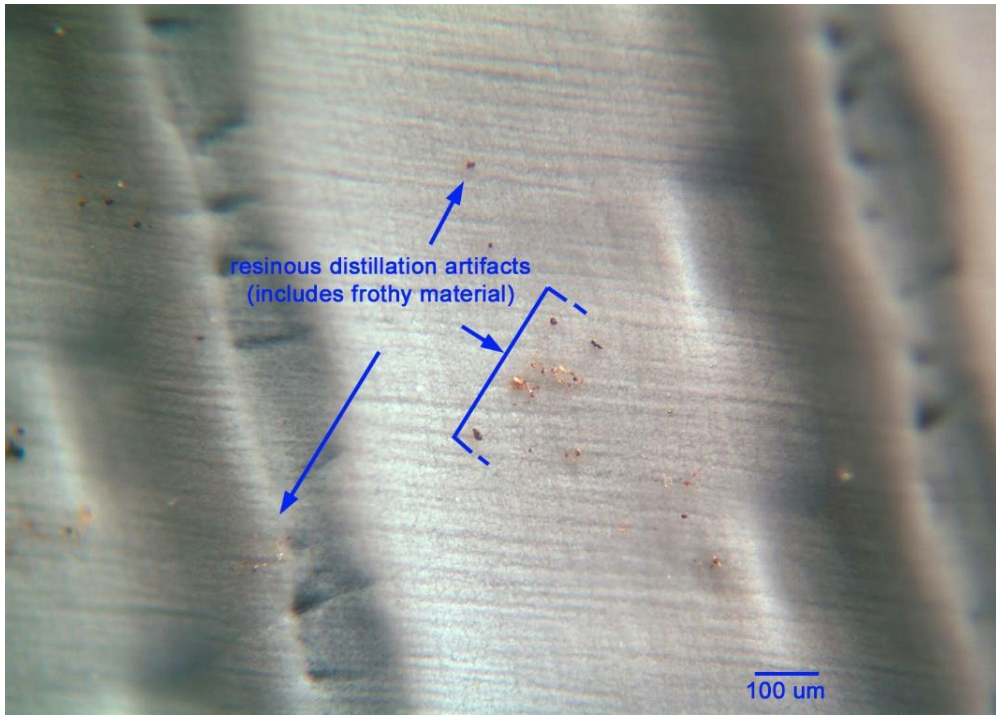
Figure 31: CFU108 Run 3 particle assemblage. These distillation-like particles may also possess iron oxide/hydroxide components, and may represent corrosion blisters.
