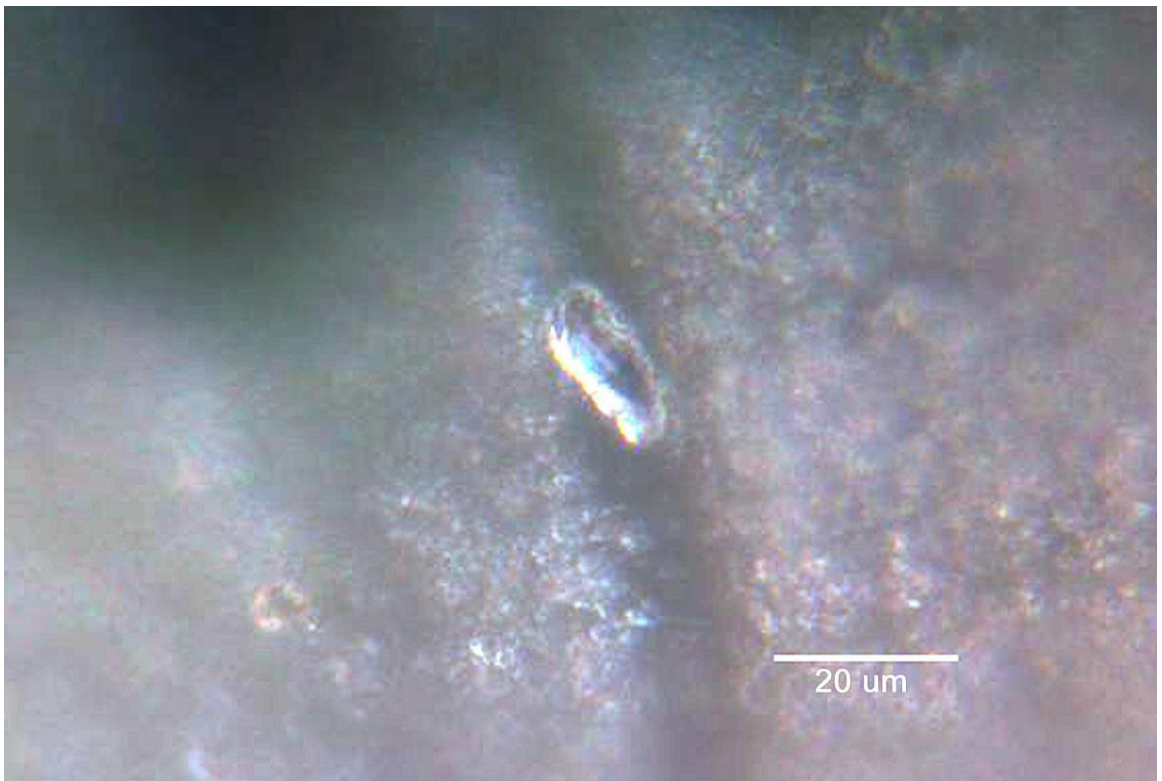
Figure 6: CFU108 -R1 showing a \sim 20 \mu\text{m} vitreous glass shot-like particle. A second smaller glass shot-like particle is also seen in the lower left.
