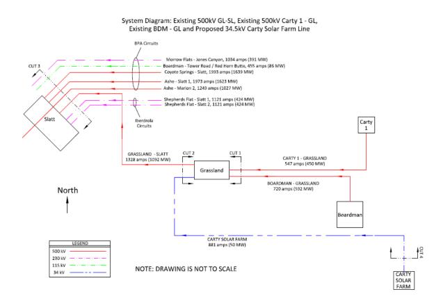
Figure AA-1 System Diagram
