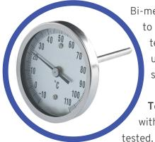
Bi-metal thermometers (as shown in the picture to the left) are not designed to measure the temperatures of thin foods, and can only be used for foods like soups, roasts, or tuna salad.
