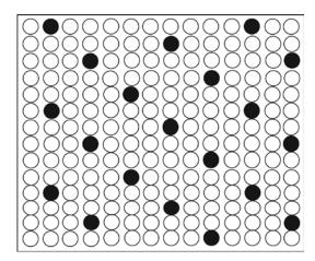
Figure 26. Systematic sample taken by selecting a starting point at random and the sampling every 10th sampling unit from left to right, wrapping around when necessary. This sampling plan preserves the same probability of a unit being selected as a simple random sample.
