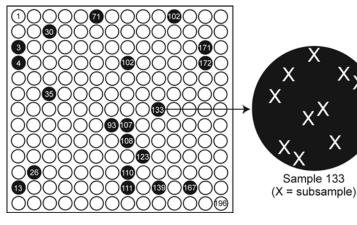
Figure 23. Subsampling: 20 random samples with subsampling within each sample. The 15th sample (Sample 133) shows ten randomly selected subsamples marked with Xs within it. In our example of potted ornamental plants (Figs 20 and 22), the subsample might be ten leaves selected at random from the plant. Although the sample contains ten subsamples, the sample itself counts as only one sample.
