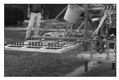
Experimental sprayers, such as this one, must be calibrated prior to being used in an experimental setting. Photo courtesy of Mike J. Weaver, Virginia Tech, http:// pesticidepics.org.
