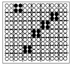
Figure 28. Cluster (area) sample: 20 samples are selected by randomly selecting five clusters of four sampling units from a total of 49 clusters and then sampling all four units in a cluster.
