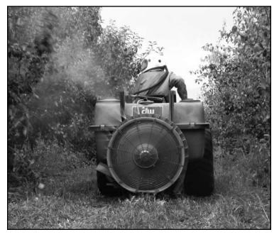
Experimental pesticides applied with an airblast sprayer. Photo courtesy of Laurie Gordon, ODA.
