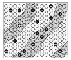
Figure 25. Stratified random sample with equal sample numbers taken from light (-) and dark (+) sections of the field (sampling strata).
