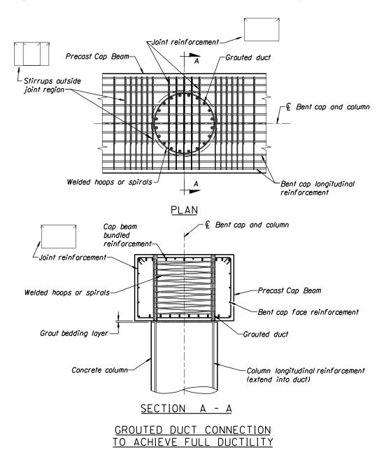
Figure 2.2.9-1 Grouted Duct Connection to Achieve Full Ductility
