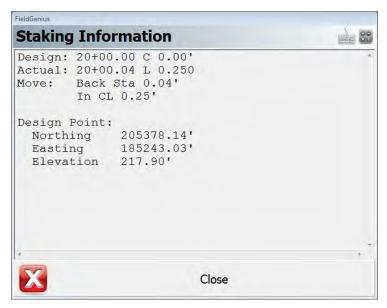
To move to the next Station without storing a shot at the current Station – tap the <u>Close</u> button on the Staking bar and the Stake Alignment menu will popup allowing you to select another Station and Offset to stake.
