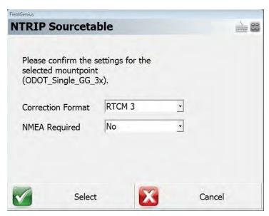
You should now be connected. If you are outside and receiving enough GNSS signals you should have an RTK FIXED solution.
