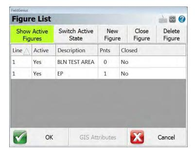
• If you want to switch to and add additional points to a different line, highlight the line you want and tap OK. It will make the highlighted line the active line.
