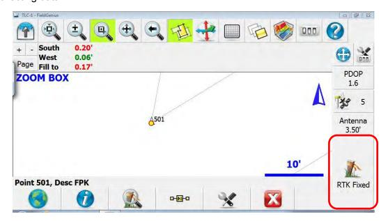
If you aren't using the external antenna, the constructed point is not exactly per plan or the point has been disturbed (moved) you will get a tolerance exceeded error. You can still tap <u>Save Point</u> and <u>Raw Data</u> to collect the point.
